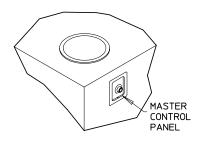
MOUNT APPLIANCE SO THAT THE CONTROL PANEL IS LOCATED TO THE FRONT OF THE FIXTURE.
